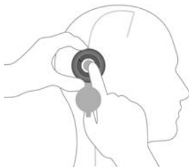
Figure 11: Adjustment using the M.blue plus Adjustment Ring
