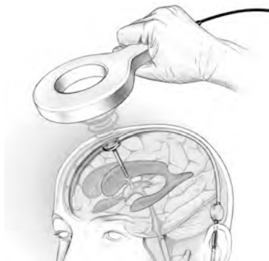
Fig. 2: The working distance for telemetric data transmission, i.e. the distance between the antenna and the M.scio is 10-30 mm
