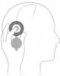
Figure 6: Localising the valve using the M.blue compass
