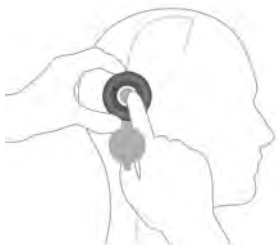
Figure 11: Adjustment using the M.blue plus adjustment ring
