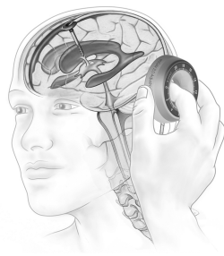
Joonis 7: Seadistamine kohandusinstrumendi proGAV 2.0 Adjustment Instrument abil
