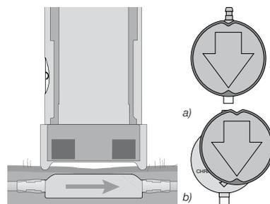
Fig. 13: Verifying the pressure setting
