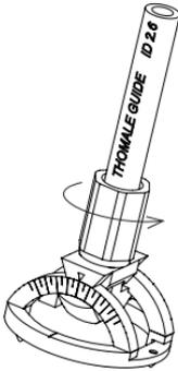
Fig. 10: Angle adjustment on the *THOMALE GUIDE*
