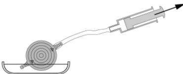
Fig. 19: Patency test
