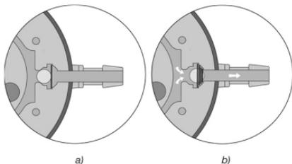
Fig. 2: Operation of the differential pressure unit
