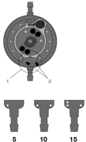
Fig. 6: Pressure ratings encodings of the differential pressure unit
