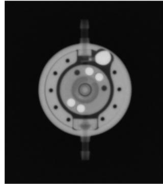
Fig. 5: X-ray image (adjustable gravitational unit preset to 20 cmH<sub>2</sub>O; differential pressure unit: 5 cmH<sub>2</sub>O)
