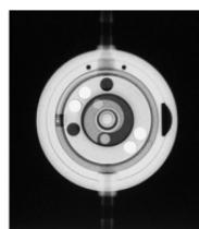
Fig. 6: X-ray image of an adjustable differential pressure unit, setting 14 cmH<sub>2</sub>O
