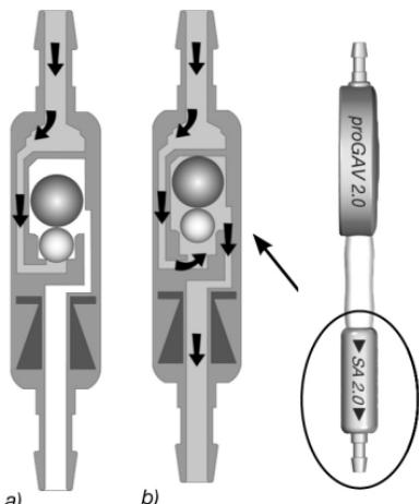
*Fig. 4: Gravitational unit in vertical body position*
