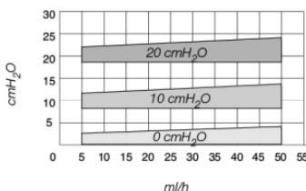
Fig. 17: Pressure flow characteristics for selected pressure levels of the adjustable differential pressure unit
