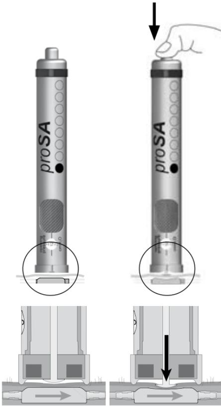
Abb. 11: Adjusting the pressure setting
