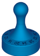
Fig. 20: M.blue Checkmate , colour: blue Pressure levels: 0 to 40 cmH 2 O
