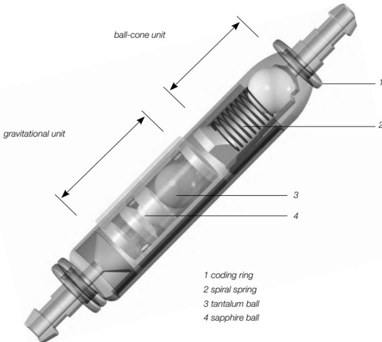
Fig. 1: Schematic cross section of the paed/GAV
